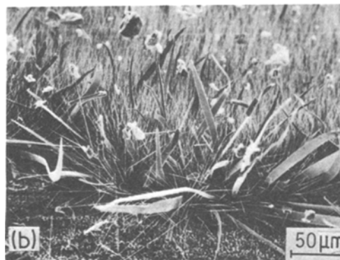
Figure 2 Appearance of pillar-like crystals grown with Au impurity. Temperature: 1220° C.
